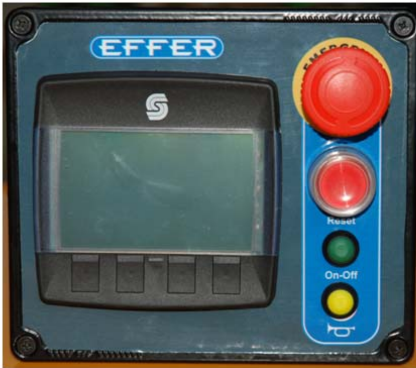
Wide display fitted on the crane
